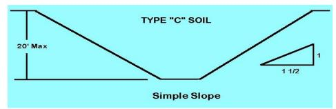
the trench would be sloped at a 34-degree angle, or 15 feet back in both directions for at least 30 feet across, plus the width of the bottom of the trench itself. All simple slope excavations 20 feet or less in depth shall have a maximum allowable slope of 1 1/2:1.
