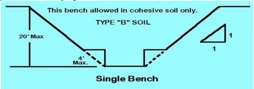
All benched excavations 20 feet or less in depth shall have a maximum allowable slope of 1:1. In Type B soil, the vertical height of the benches must not exceed 4 feet. Benches must be below the maximum allowable slope for that soil type. In other words, a 10-foot deep trench in Type B soil must be benched back 10 feet in each direction, with the maximum of a 45-degree angle.
